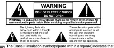
this product has been evaluated and tested to comply with Class II insulation requirements.
